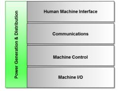
Alongside these four ingredients is the power generation and distribution system, often 12 or 24VDC supplied initially by 110/220VAC wall power.
